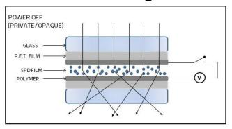
Solar SmartGlass™ is a solar control glass. When an AC electrical current is passed through the glass it instantly changes from darkened to visibly clear state. When the electrical current is removed it returns to the darkened "private" state in less than 10 seconds.
